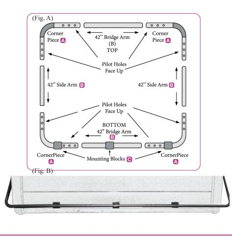
5. Next connect these two assembled pieces together with the Side Arms (B) by sliding the Side Arms into each of the four Corner Pieces as shown in Fig. A DO NOT secure with screws yet. With the Spa Cover in place on your Spa, lay the assembled rectangle assembly on the spa with the Mounting Blocks at the bottom as shown in Fig. B. Remember, screws face up as shown in Fig. A.
