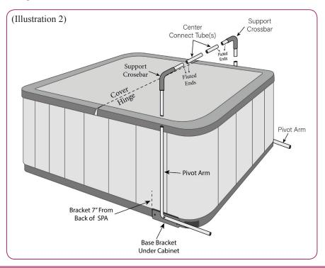
4. Insert the LONG end of the Crossbar Support Arms (Part C) into the Pivot Arms (Part B). Next, use the non-fluted Center Extension (Part D) to connect the Support Crossbar Arms (Part C). To add length for spas over six feet, add the fluted Center Extension (Part D). See Illustration 3.
