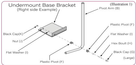
3. SLIDE both Under Mount Base Brackets under the spa with the Pivot Arms (Part B) in the upright position. Note: The edge of the Base Bracket should be 7" from the edge of the spa. See Illustration 2 & 3.
