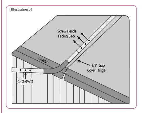
5. Lay the assembled Lifts on the closed spa cover. Adjust Support Crossbar Arms (Part C) & Center Extensions (Part D) so that the side of Support Arms are approx. 1/2" away of the center of the cover fold.
