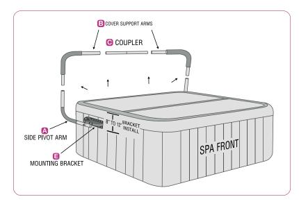
2. Connect the Pivot Arm (A) and two Bushings (D) to the Mounting Brackets (E), using one  $3/8" \times 3"$  Hex Cap Bolt (F), two 3/8" Flat Washers (H), and one 3/8" Nylon Locknut (G).REPEAT
