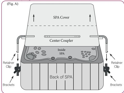
3. Attached the Left & Right Mounting Brackets Assembly to the appropriate side of the Spa Cabinet (using  $\#10 \times 1$  mounting screws) Brackets must be fitted underneath the
