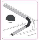
9. You may add the Towel Hook at this stage, using #10x 5/8" screws. Install on the black screw head domes. A small amount of glue/epoxy will help secure domes.
