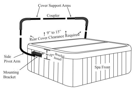
2. Connect the Pivot Arm (A) and two Bushings (D) to the Mounting Brackets (E), using one 3/8" x 3" Hex Cap Bolt (F), two 3/8" Flat Washers (H), and one 3/8" Nylon Lockwet (G) PEPEAT.
